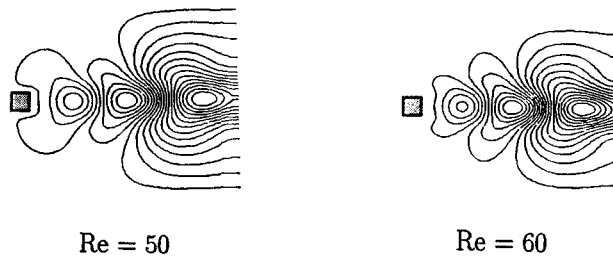
Figure 5. Instantaneous streamlines of the most unstable perturbation to the steady flow at Re=50 and 60
